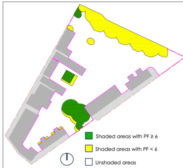
Figure 4.6: A shade protection factor map of the study school, showing the shaded areas with and without the required protection factor rating
